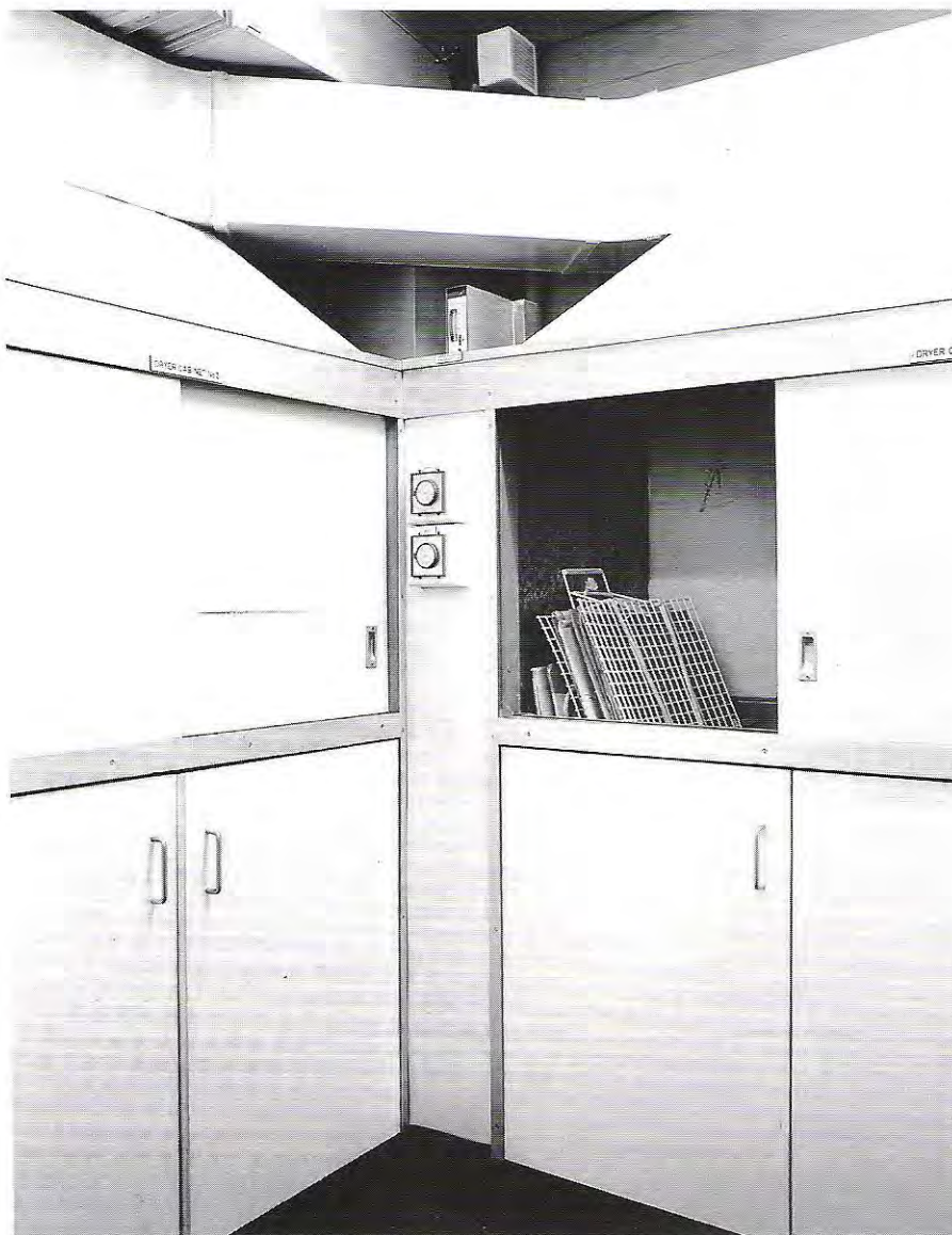
Figure 3.2 Drying cabinets with a forced circulation of warm air, as used in large herbaria to shorten drying time and to lessen the need to change drying papers.
