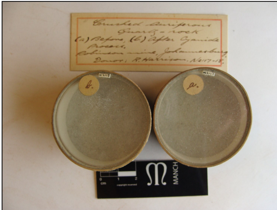
Figure 5. 'Crushed auriferous Quartz-rock (a) before (b) after Cyanide process' Robinson Mine (MANCH-N.2117 and MANCH-N.2118), donated by R. Harrison, accessioned 1914. © Manchester Museum, University of Manchester.
