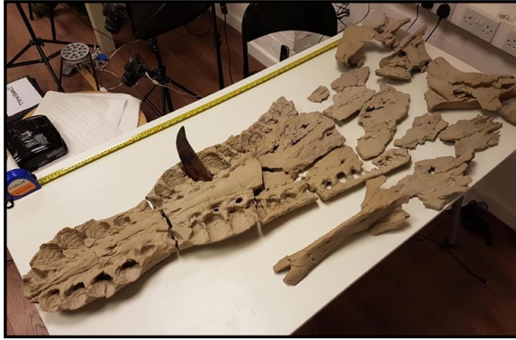
Figure 10. All the pieces of the pliosaur skull freshly 3D printed in gypsum at ThinkSee3D (with a single replica tooth placed temporarily in a socket). Image credit: SD.
