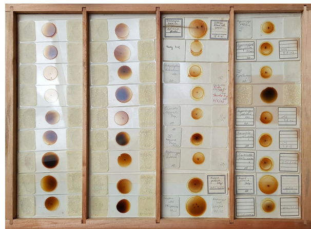
Figure 2. Slide drawer showing discolouration of Canada balsam mounting medium due to the presence of paradichlorobenzene in adjacent historic insect cabinets. Note that the intensity of the discolouration is greater in slides that have not been sealed. Image © Paolo Viscardi, 2018
