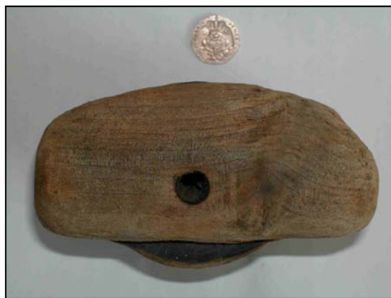
Fig. 4d. Composite pulley block. a, b waterlogged as found; c, d air dried after prolonged immersion in aqueous sugar solution
