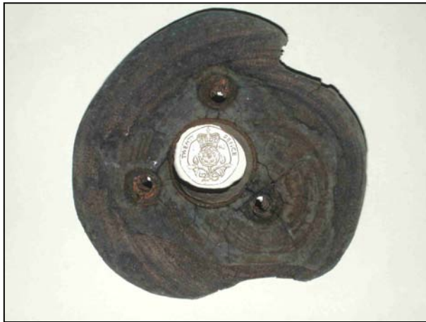
Fig. 1. Air dried, lignum vitae ( Guaiacum ) sheave from the English Channel.. (Scale: 20p UK coin, 21 mm diameter)
