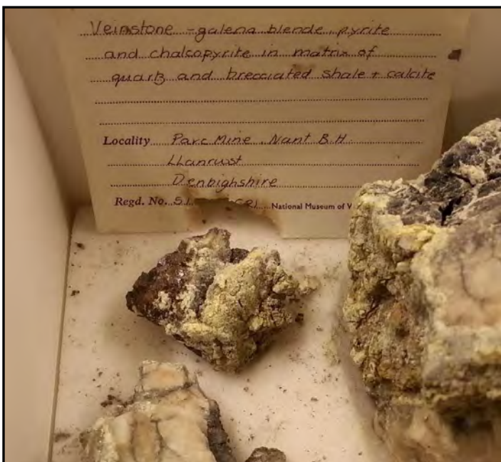
Figure 3. Image of a veinstone specimen affected by pyrite decay. Part of the specimen has spalled off. All parts feature characteristic yellow and white sulfate efflorescence. Also note the 'scorching' of the label caused by sulfuric acid, which has defaced the accession number, potentially resulting in dissociation of specimen and contextual information. Image National Museum Cardiff.
