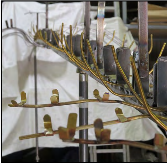
Figure 5. Brass strips and rods brazed together to hold smaller ribs in place. Image credit: NRL.
