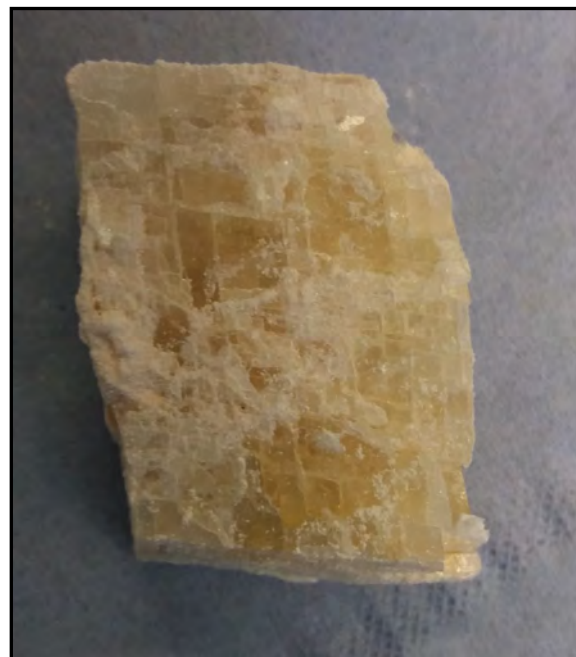
Figure 4. A calcite ( \text{CaCO}_3 ) sample displaying spalling, cracking, and efflorescence following exposure to acetic acid within severe accelerated aging conditions.
