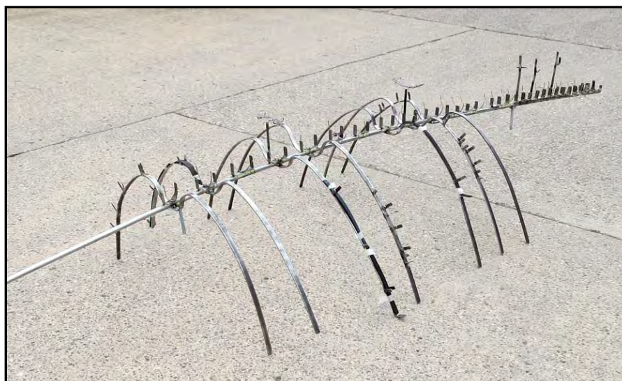
Figure 4. The steel frame made to hold the larger ribs and vertebrae in place, not yet positioned on the upright supports. Image credit: NRL.
