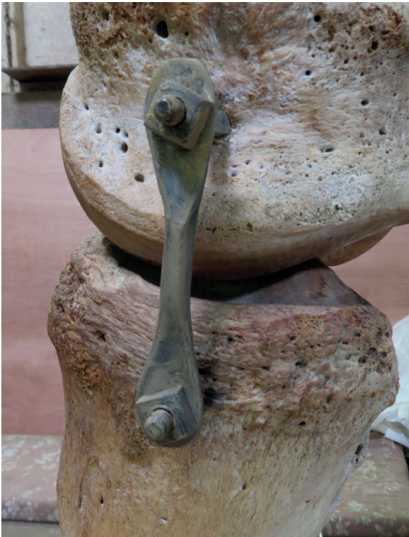
Figure 10. One of the five brackets made on the forge to hold the lower limb bones in articulation with the upper limb bones. Image: Nigel Larkin.
