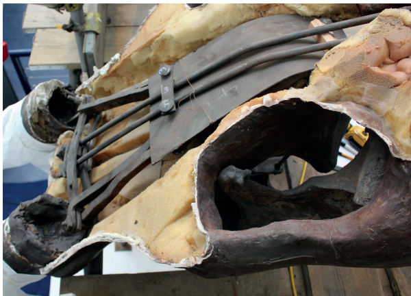
Figure 3. The Victorian armature inside the skull cast, which links the tusks to the torso. Image: L.Allington-Jones, © The Natural History Museum.
