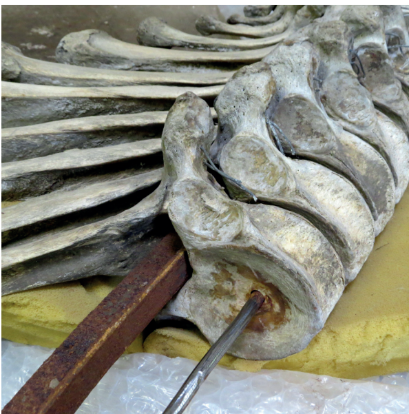
Figure 6. The rusty T-shaped vertebral bar with some of the vertebrae still attached. The thin vertebral rod has been cleaned in an attempt to remove it from the vertebral centra. Image: Nigel Larkin.
